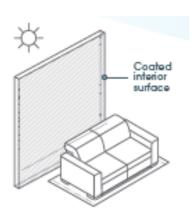
Low E coated glass has a very thin metal coating on the interior glass surface. This hard and durable coating gives the product its improved thermal insulation and solar control performance compared to ordinary clear glass. The coated surface of the glass does clean differently to ordinary glass and these guidelines are recommended for the most appropriate hand cleaning results.
